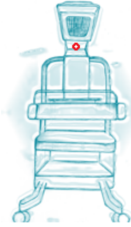
Fig. 1. Schematic showing the optimal mount position for a camera in a warmer (red dot)
